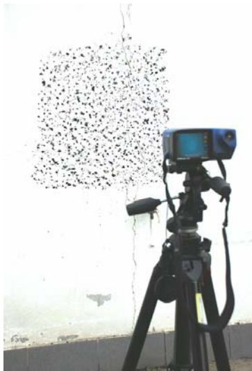
Fig.5. The photo of experimental setup with DICIR sensor.
